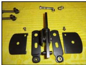
Since this is a solid design, we can accommodate both with minor adjustments. So let's make the tower bracket to fill that 3-1/4" by 1-1/2" hole you labored over in the top plate. Using 10 gauge steel. Cut out two pieces that are 3 inches by 4 inches. The hardest part of this procedure is trying to get the center hole at the proper height for the lower mechanism to meet up properly. There are two issues we are concerned with here. One is proper
