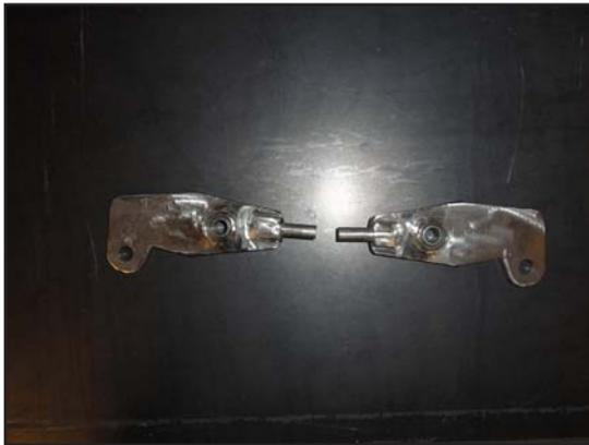
They must be opposing each other and have the rod protruding upward on the proper side. The protruding rod must be 3/4" and be cleanly welded so that the entire 3/4" can be used. Now that you are ready to weld, clamp the rod down to the table as well as the pivot so its positioned correctly and go for it!
