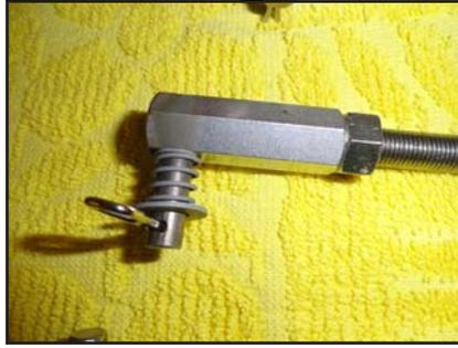
Weld the 5/16" rod by placing weld inside that end of the coupling nut. Pretty solid way to hold the rod in. Sometimes things just work out! Now, cut three pieces of 3/8"-24 all thread that is as follows:
